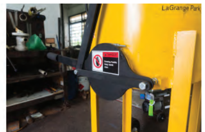
Slide gate for easy discharge
