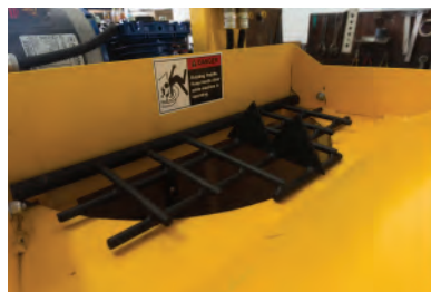
Built-in bag breaker for easy material loading
