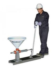
The heavy-duty Model CG-050M is an easy to use, skid mounted hand pump designed for smaller jobs using high viscosity slurries and most pre-packaged grouts. Its rugged, lightweight aluminum construction offers mobility in areas where no air or electric power sources are available.
