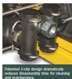
The ChemGrout High Pressure Pump series are skid mounted grout pumps. These low maintenance pumps are designed to work with your grouting batch plant or mixing system. The grout pump is a double acting, positive displacement, plunger style pump. The plunger pump is designed so that conversion between the pressure outputs is quick, easy and cost effective.
