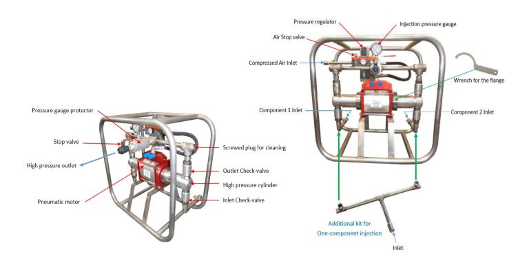
The Pro35 portable grout pump is an air-driven, double acting piston pump specially designed for injection of cement slurry, bentonite mud, water and also for two components injection. This pump's light weight and compact dimensions make it ideal for use on work-sites where space restrictions make it extremely difficult or impossible to use heavier equipment.
