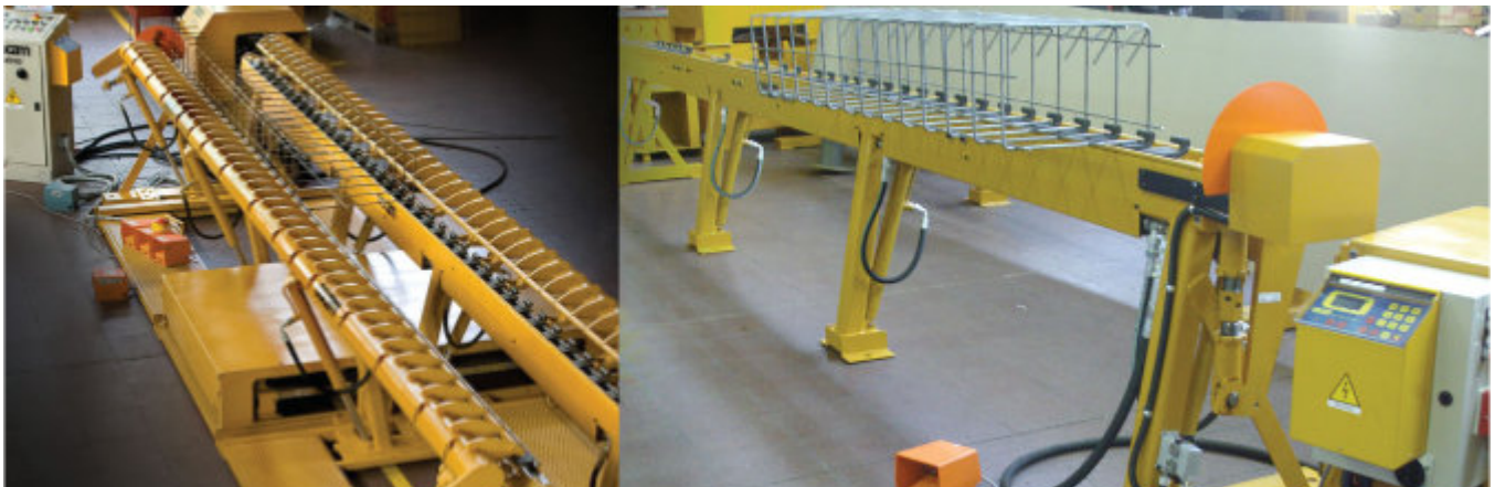
Mesh Bending Machine
