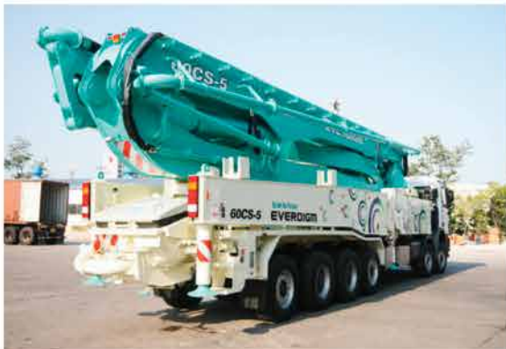
Truck Mounted Concrete Pumps
