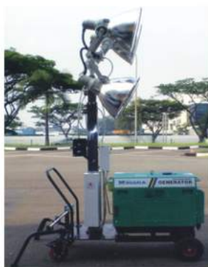
Generator with flood lights
