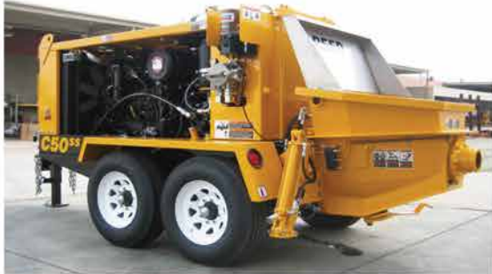
Stationary Concrete Pump
