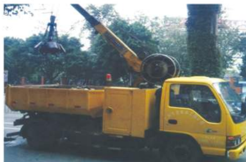
Trucks for Drain Works
