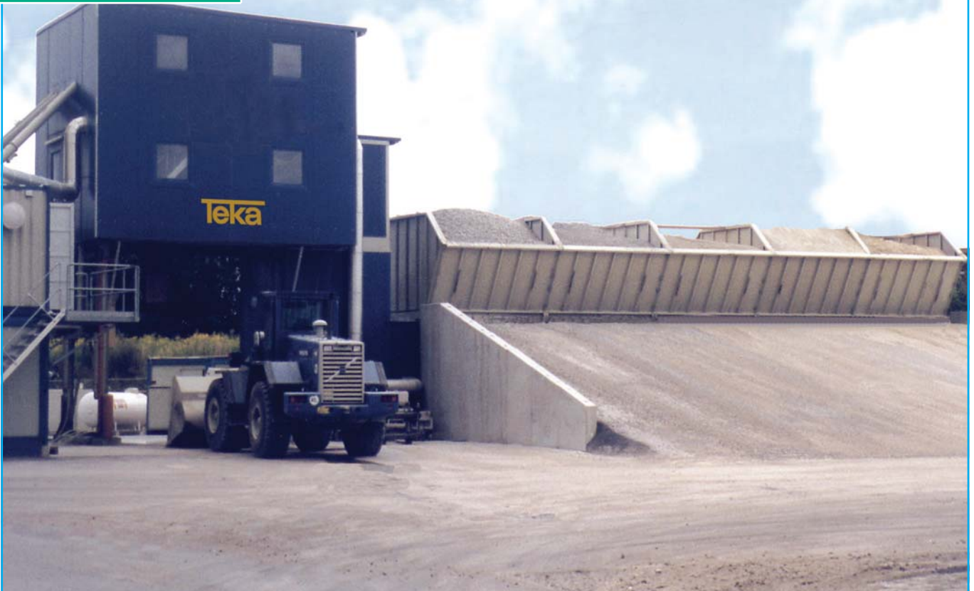
MIXOMAT THZ 3000 C - R 5 / 5, Reihen-Siloanlage, 5 Kammern • MIXOMAT THZ 3000 C - R 5 / 5, aggregate in-line silo system, 5 compartments
