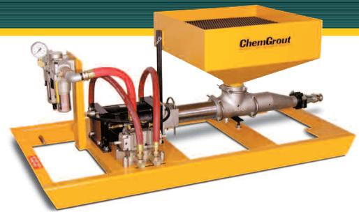
Complete grouting systems combine the CG-030 piston pump with a high efficiency paddle mixer to provide a continuous output of material. Both mixer and pump are equipped with their own variable speed control.
